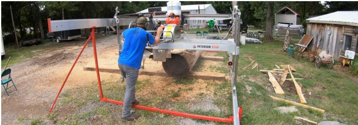
As somewhat of a salvage revivalist, Matt often comes upon odd-shaped or extra-large logs which can’t be cut with most bandsaw mills. With a bandsaw’s style of cutting, large logs require turning until the end is in the shape of a ‘stop sign’, whereas Peterson’s design allow the sawyer to tackle large logs head-on.
