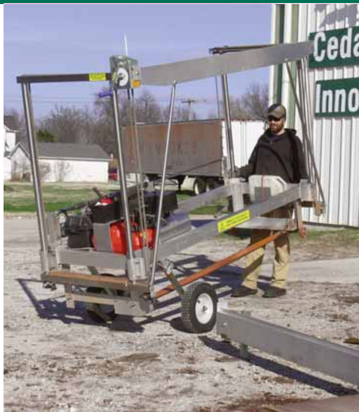
Jesse rolls out the cutterhead for his Peterson slabber. The entire assembly rolls onto the tracks with no heavy lifting. In about 10 minutes, he was ready to cut.
