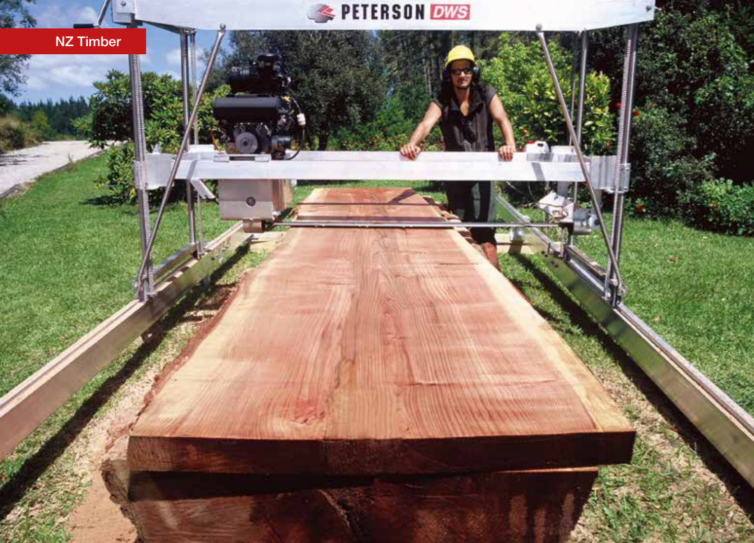
Above: The Dedicated Wide Slabber cuts logs into high-value wide slabs using a chainsaw slabber style bar.
