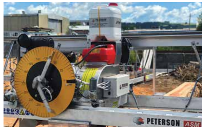
Below: Close-up of the main carriage of the Automated Swingblade Mill (ASM). The ASM makes horizontal and vertical cuts, changes the size or depth of the cut, and removes the previously cut board, all at the touch of a button by the operator.
