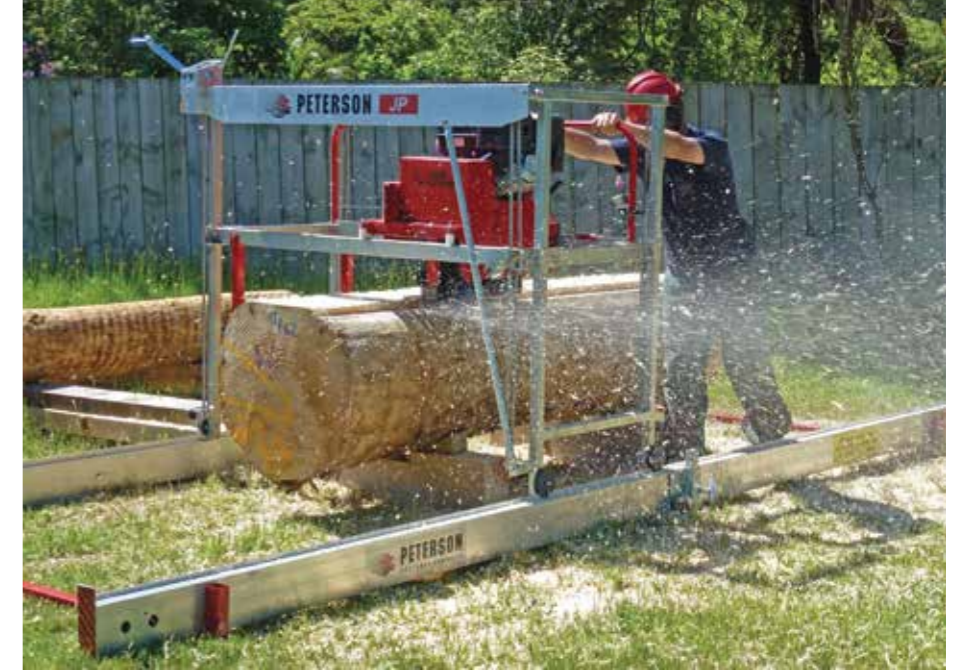
Right: The Junior Peterson is the perfect swingblade sawmill designed for part-time sawmilling.
